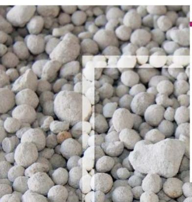
Due to its extremely high anhydrite content and the minimum concentration of impurities, the quantity of SO<sub>3</sub> per tonne of material is the highest compared to the other natural or chemical gypsums. Its use therefore allows a reduction in specific consumption of calcium sulphate based raw materials used in the production of cement.
